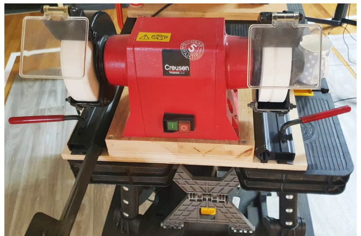
Bench grinder fitted with white Aluminium Oxide wide wheels, the One Way jigs can be seen in the left and right on the base plate
