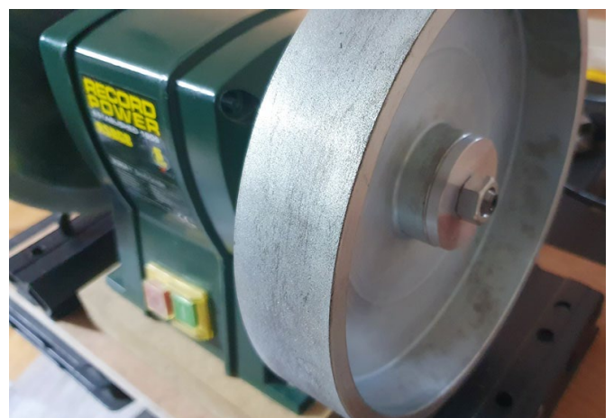
Above: Record power 6 inch bench grinder fitted with two grades of Cubic Boron Nitride (CBN) wheels
